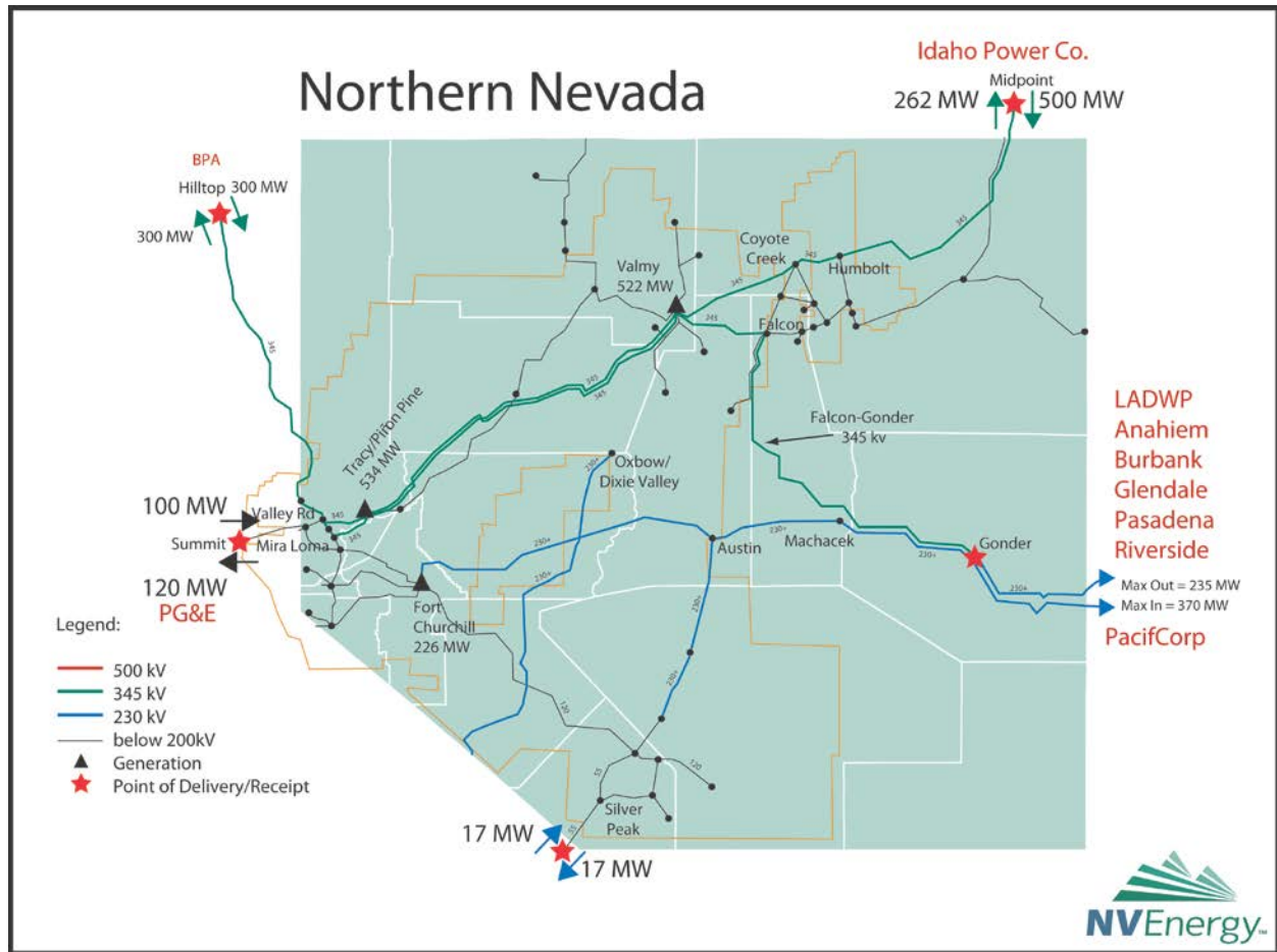
Figure 3-1 NVEN Transmission System
